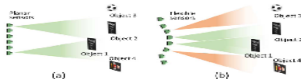
Fig. 1. (a) Illustration of a conventional integral imaging system where sensors are on a planar surface. (b) A flexible sensing integral imaging system where the sensors can be placed on any arbitrary surface.
